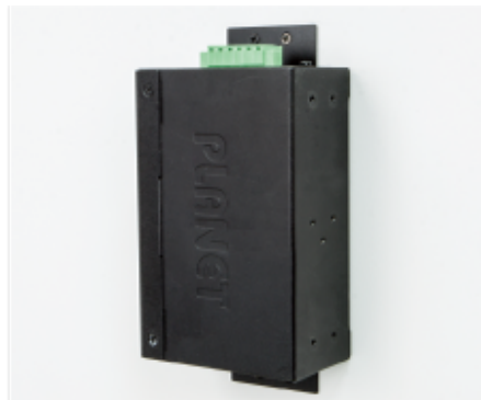
Side Wall Mounting (Space saving)
